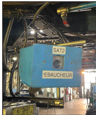
Equipped with Near-Infrared (NIR) cameras for early fire detection and mechanical jam alerts
